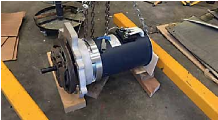
Motor with assembled spacer, adapter and clutch in place. I still needed to make a front motor mount.
