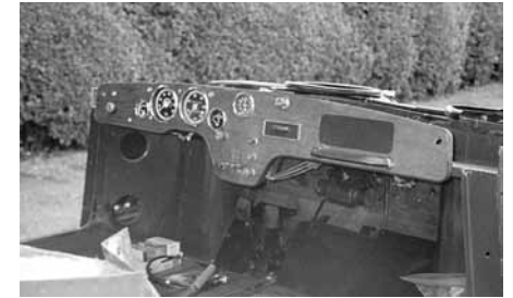
Original dashboard, sometime in the past someone had fitted a later temperature gauge; the hole is now too big to fit the original sport/M.C. type.
