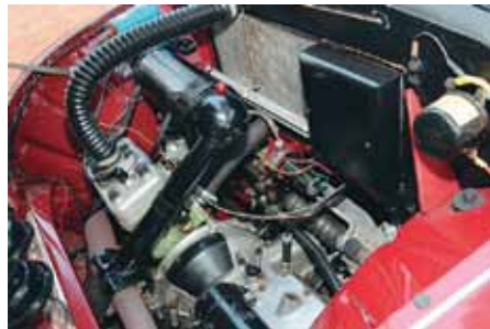
92B powered by 764cc water-cooled two-stroke engine
