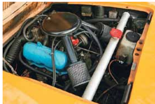
Tiny bonnet reveals Ford V4 engine – good for 170km/h performance
