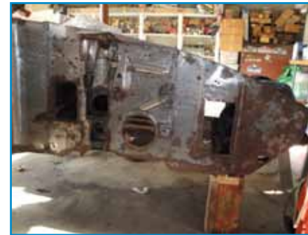
A stripped wheel well reveals all the rust.
