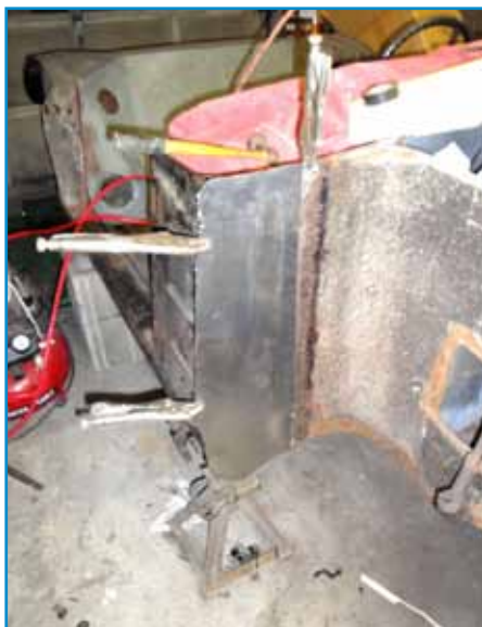
New patch ready to be welded in place.
