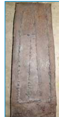
LOL! 4 pieces of scrap metal was used to repair the rear wheel well.
