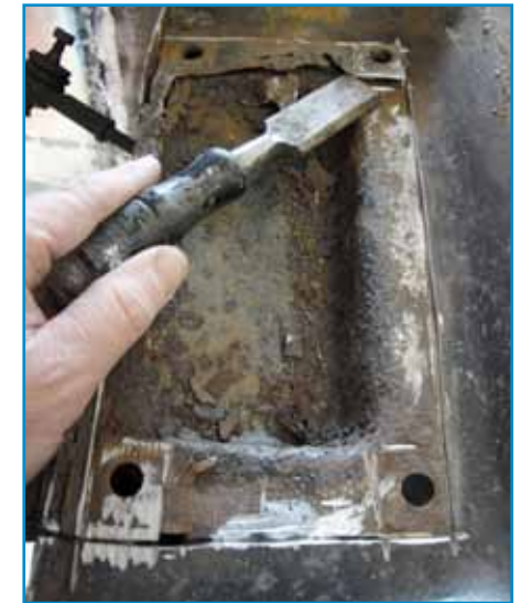
Carefully opening up the lower "A" arm attachment.
